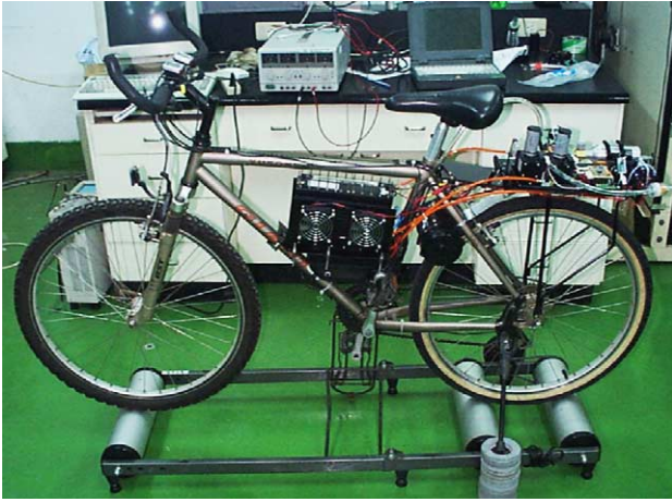
Fig. 5. Roller-stand test of fuel-cell bicycle.
