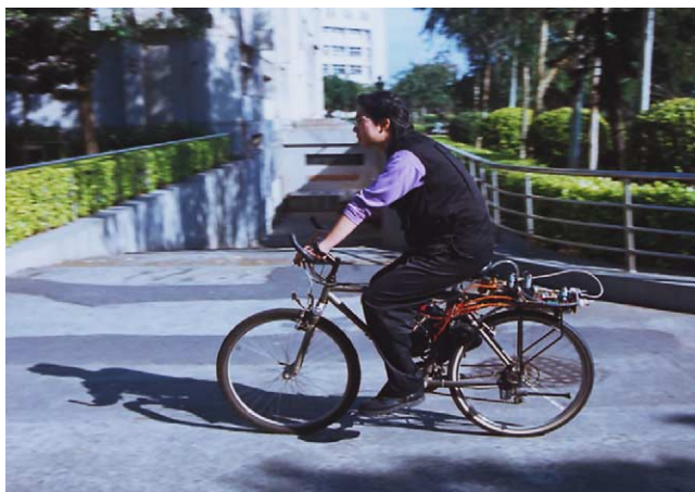
Fig. 6. Road test of fuel-cell bicycle.
